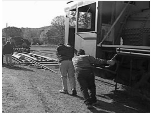
Roller bearings and a down-grade work wonders in moving loco to where a tow cable can reach it.
