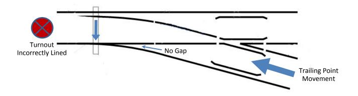
A trailing point movement through an incorrectly lined switch likely results in one or two very undesirable outcomes:
