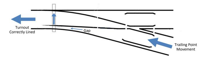
A turnout incorrectly lined for a trailing point movement lacks the gap needed for the passage of the wheel flanges.
