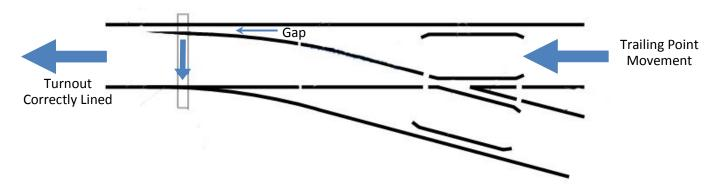
A turnout correctly lined for a trailing point movement provides a gap at a location necessary for the passage of the wheel flanges along the inner (or gauge) side of the stock rail.
