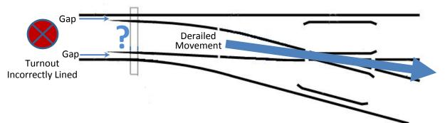
A facing point movement made over a turnout in this condition will be derailed, landing in the middle of the two possible routes. This mistake is known as "**Splitting the Switch**".
