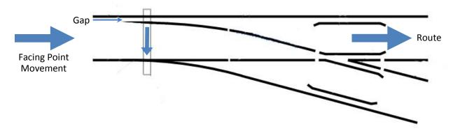
A rail vehicle making a facing point movement will be directed towards the side of the turnout where there is a gap between one of the point rails and its companion stock rail. If the turnout is not properly lined, a rail vehicle making a facing point movement will end up on the wrong track.
