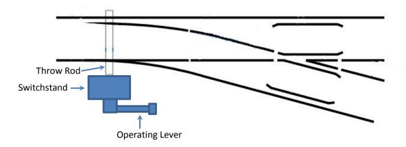
When a rail vehicle is moving toward a turnout from the side of the points, this movement is called a "**Facing Point**" movement. A facing point movement is one where there is a choice of route based on the position of the points.
