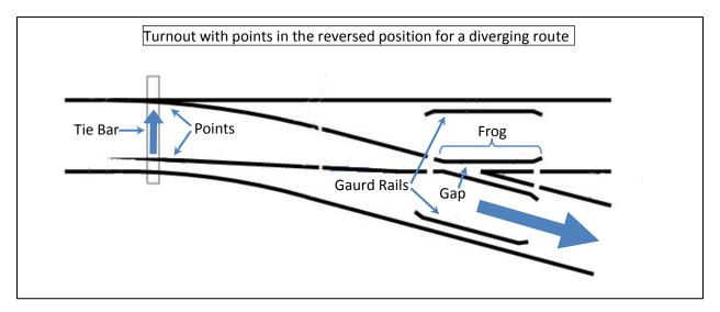
Turnouts have a stationary section called the "**Frog**" which contains a gap at the point where the rails for the two different routes cross each other. This gap creates a clear path for the wheel flanges to pass through. The frog works together with the "**Guard Rails**" to ensure the wheels follow the correct path through the gap.
