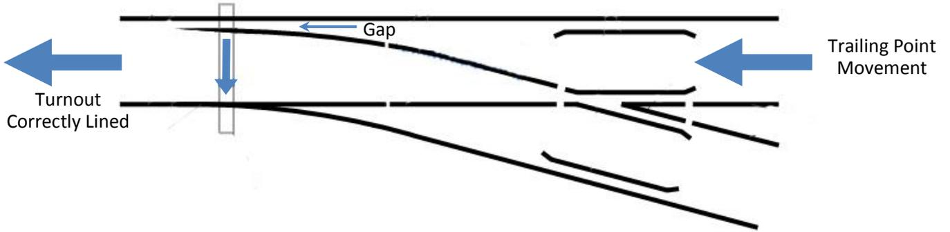
A turnout correctly lined for a trailing point movement provides a gap at a location necessary for the passage of the wheel flanges along the inner (or gauge) side of the stock rail.
