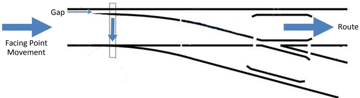
A rail vehicle making a facing point movement will be directed towards the side of the turnout where there is a gap between one of the point rails and its companion stock rail. If the turnout is not properly lined, a rail vehicle making a facing point movement will end up on the wrong track.
