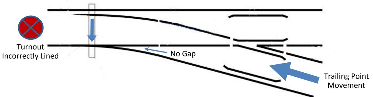
A trailing point movement through an incorrectly lined switch likely results in one or two very undesirable outcomes:
