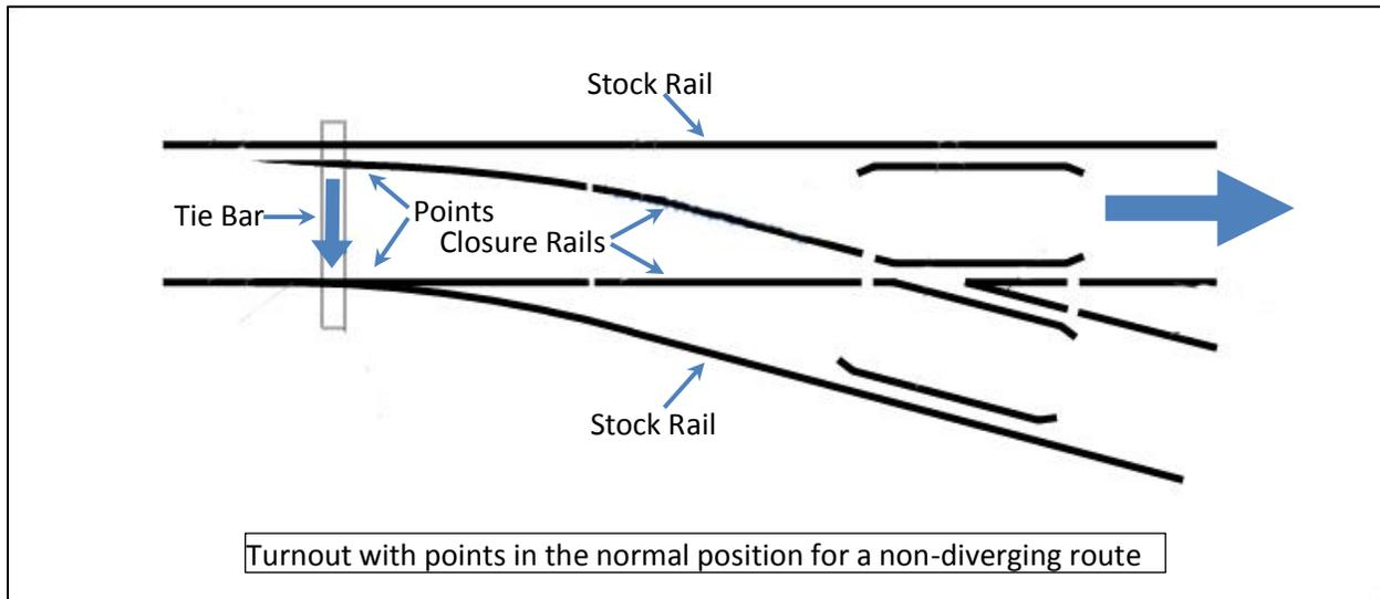
Turnouts have moveable sections of tapered rail called “**Points**”. Each turnout has a set of two points joined by a “**Tie Bar**”. The tie bar moves the points move back and forth together. The position of the points determines which route the turnout is set, or “**Lined**” for, i.e. the route a rail vehicle will take when passing through the turnout.
