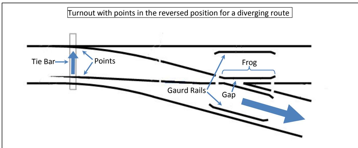
Turnouts have a stationary section called the “**Frog**” which contains a gap at the point where the rails for the two different routes cross each other. This gap creates a clear path for the wheel flanges to pass through. The frog works together with the “**Guard Rails**” to ensure the wheels follow the correct path through the gap.
